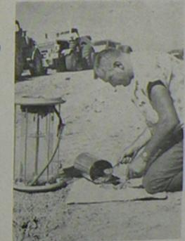
Checking compacted fill for density determination with water-balloon method, a typical step in testing and control by Engineers Testing Laboratories, Inc.
